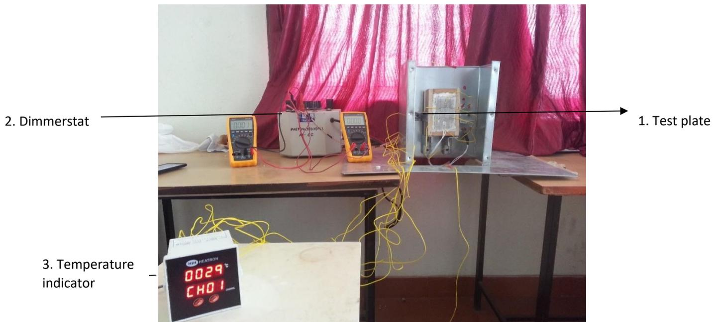
Figure 1: The experimental setup.
