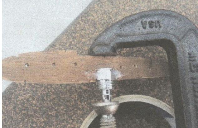
Fig. 4: Air hose connector attached at the lower surface of the airfoil.
