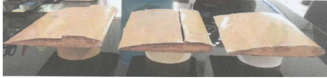
Fig. 3: Three side views of the airfoils.
