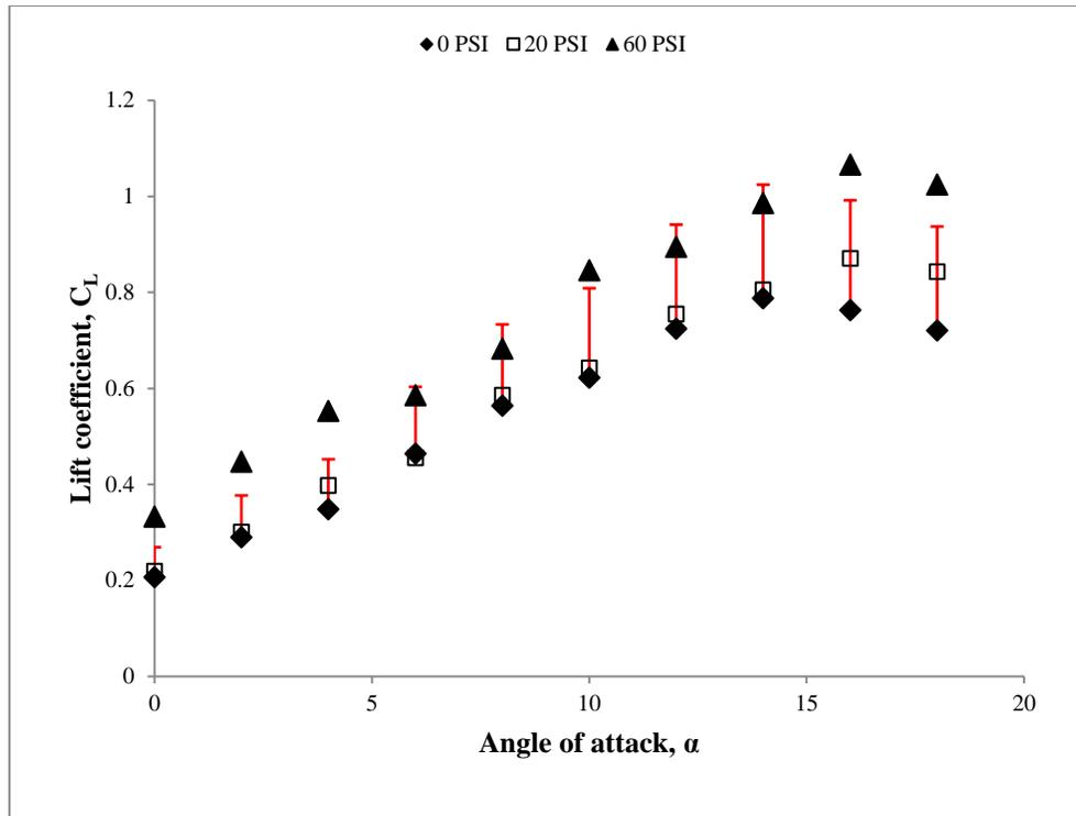
Fig. 6: Lift coefficient versus  $\alpha$  for Reynolds number 50 000.
