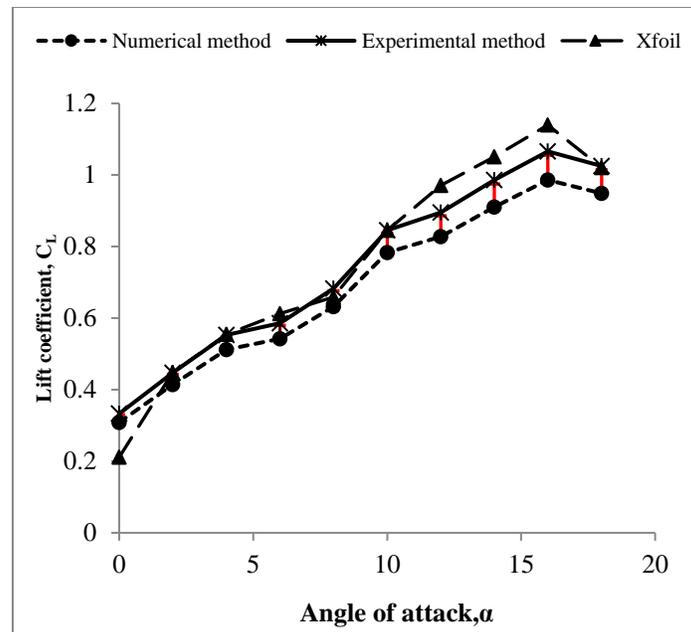
Fig. 8: Comparison between numerical method and Xfoil database.
