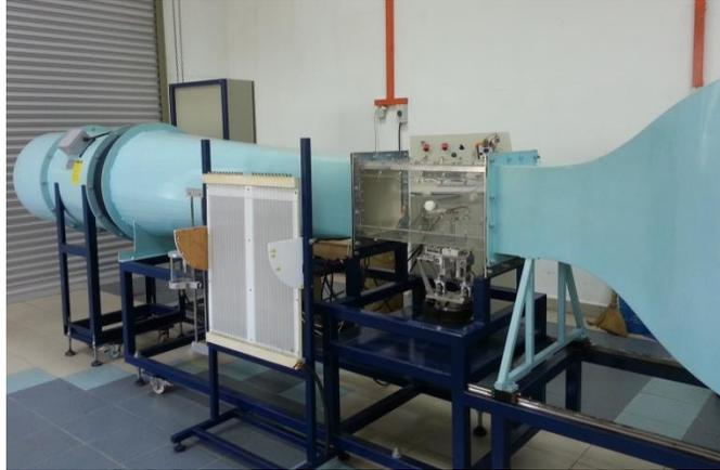
Fig. 1: The experimental setup with open circuit low speed wind tunnel.
