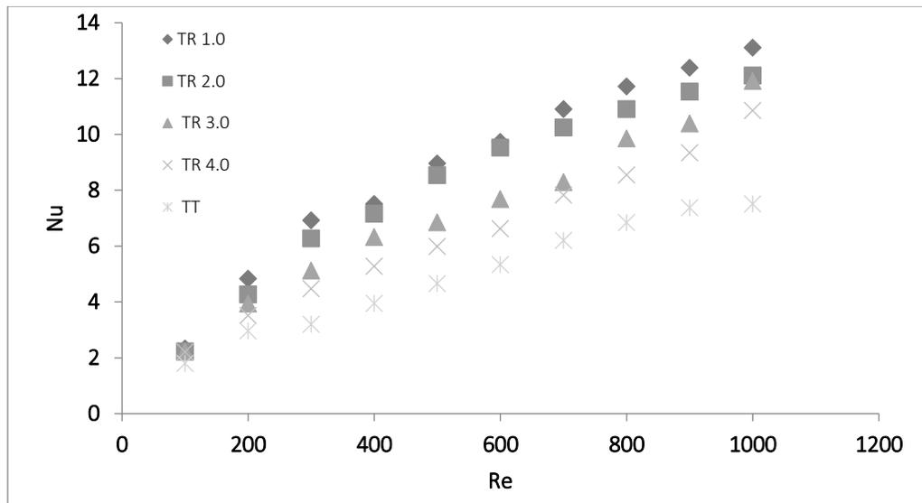
Fig. 4. Variation of Nusselt number with Reynolds number for different twist ratios.
