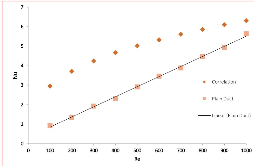
Fig. 2 Verification of the Nusselt number for the plain circular smooth duct.
