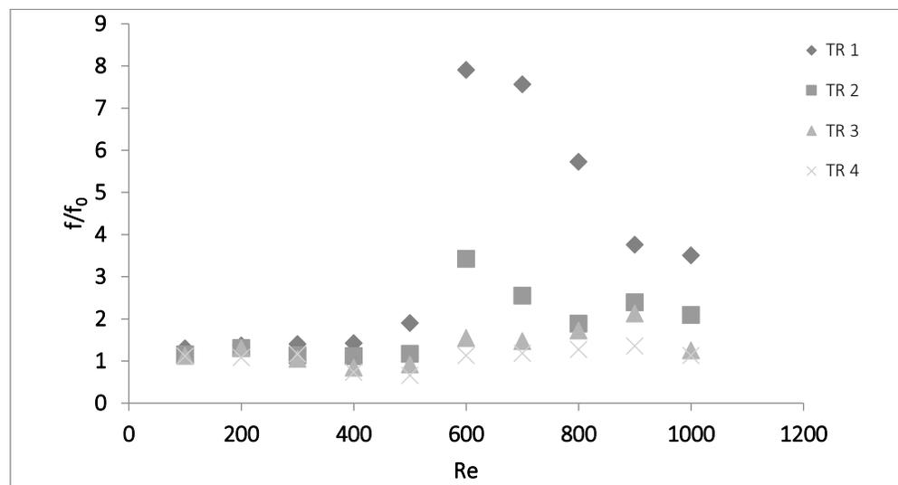
Fig. 7. Variation of  $(f/f_0)$  with Reynolds number for different twist ratios.
