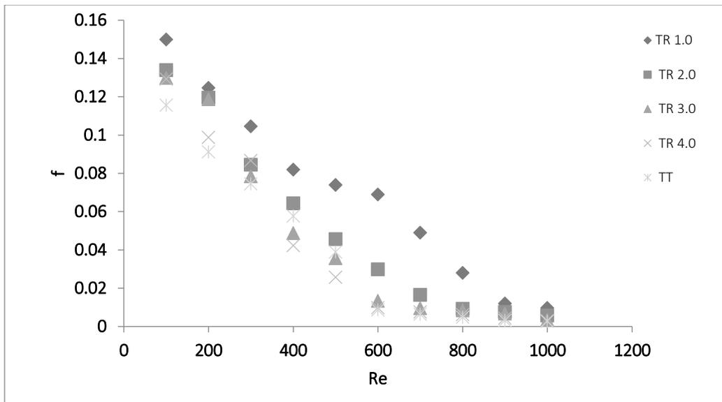
Fig. 6. Variation of friction factor characteristics with Reynolds number for different twist ratios.
