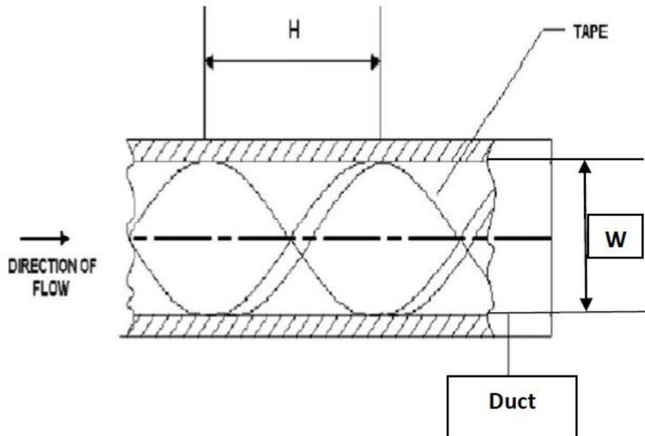
Fig. 1. Layout of the circular duct containing a full-length twisted-tape
