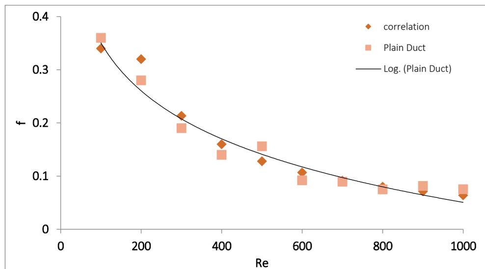
Fig. 3 Verification of the friction factor for the plain circular smooth duct.
