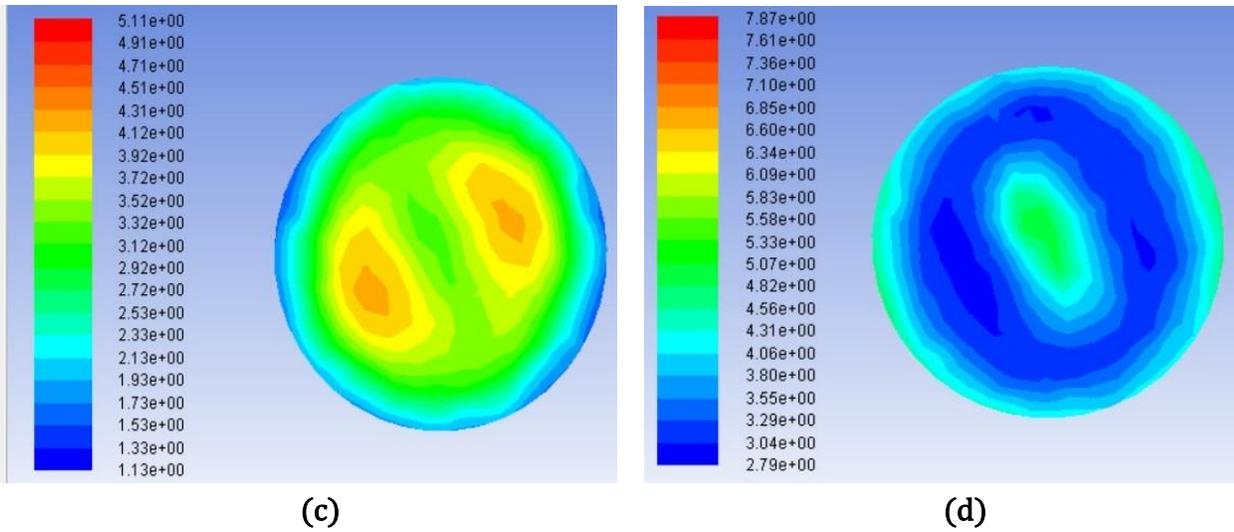
Fig. 8: X- Vorticity contours at outlet of the duct at  $Re = 800$  for different twist ratios; (a) TR 1.0, (b) TR 2.0, (c) TR 3.0, and (d) TR 4.0.
