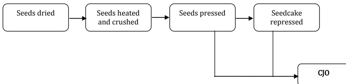
Figure 2: Crude Jatropha oil (CJO) extraction process.
