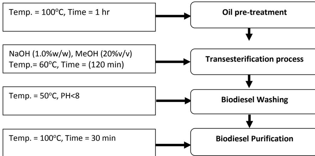
Figure 3: Biodiesel production process steps.
